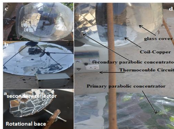
Figure1: Shows the parabolic dish concentrator with its parts: a- secondary parabolic concentrator inside of its, b- parabolic concentrator C- glass cover d- all of parts that used experimentally.
