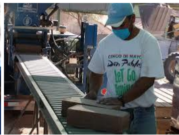
FIGURE 18. Machines produce single, a few or large number of stabilized earth bricks
