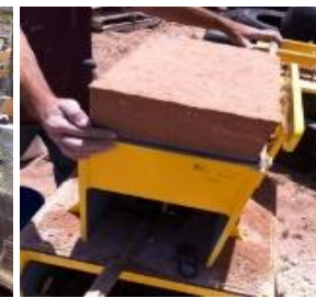
FIGURE 18. Machines produce single, a few or large number of stabilized earth bricks
