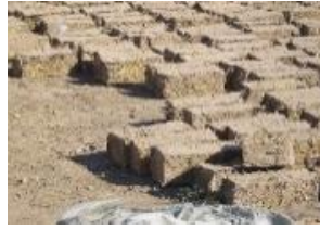
FIGURE 13. Chopped straw used as stabilizer in some areas as Saudi Arabia
